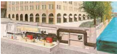
Cross section of the heat pump facility under the Walche. Photo: ETH Zurich.
